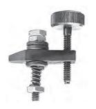
Fast-acting clamp for light-duty holding. Includes strap, knurled thumb screw, spherical washer, stud, plain flat washer, three hex jam nuts and spring. Features free swinging adjustments for positioning the assembly without interference.
