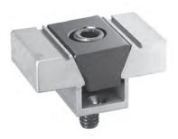
The compact Machinable Expanding Micro™ Clamp is available with extra material on the clamping jaw so it can be machined to conform to the shape of your workpiece - enabling you to fixture unusual applications easily. The specially designed steel wedge spreads the clamping force uniformly on both sides of the aluminum channel. Clamps may be ordered with a unique locking plate to make the clamp rigid while machining the jaw to your specifications, without vibration.
