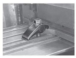
Forged Adjustable Clamp holding one side of a hydraulic vise on a milling machine table.
