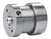
Double Acting Cylinders can be used for clamping, holding positioning, staking, punching...anywhere that a heavy duty cylinder is needed. If the cylinder is mounted in the fixture (as opposed to using mounting brackets), the fixture should be bored to between .0005 and .0010 over the "A" dimension. Doing so will prevent an out-of-round condition of the cylinder body which could damage the piston. They may be returned by air or by hydraulic pressure.
