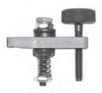
A light-duty clamp assembly for clamping close to the edge. Complete with radius strap, double jam nuts with spherical washers, finger tip, quick-action knurled thumb screw heel rest, stud, spring and washer. The latter allows free swinging and lateral adjustments for easier set-ups.
