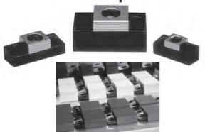
This cam action fixture clamp provides positive down force while using very little space on the fixture. Workpieces can be clamped in series by using the back surface of a clamp to locate the next workpiece. The hardened steel clamping element has both a smooth surface for machined workpieces and a serrated clamping surface for rougher work. The height of the clamp can be adjusted by milling the slot deeper in the fixture plate.
