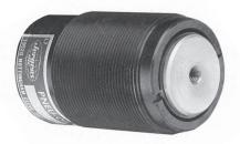
Full-threaded bodies ensure easy mounting and simple length adjustments. Their small size provides high work holding forces in tight places. Threaded Cylinders have hardened piston rods, steel bodies, alloy springs and Teflon® back-up rings which ensure trouble-free operation and long life. Not suitable for air operation. For mounting, see bracket and jam nuts on page 153.
