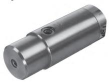
This unit is designed to be used on any machine tool with its own hydraulic system where higher pressures are needed. Jergens Intensifiers will pre-fill your circuit at approximately 200 psi maximum. Once the Intensifier sequences over to its high pressure mode, it will deliver one cubic inch of working oil at seven times the input pressure.
