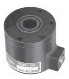
Hollow Rod Cylinders are ideal for converting existing fixtures to power clamping. Replaces clamps which use double cams, flange nuts, draw bars, or other mechanical devices. Generally, no special machining is required, just a longer stud.
