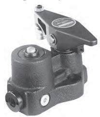
Jergens Swing Clamps are designed to swing 80° away from the workpiece to allow easy accessibility for part insertion or removal. Swing Clamps may be used in any attitude. The clamping arm may be positioned to swing either to the left or right by repositioning one cap screw. The right hand swing is standard.
