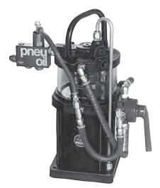
Jergens Pre-Fill Power Pacs provide a complete portable power source. Everything required to power and control your hydraulic fixture is included. Connect your shop air to the filter/regulator, and your fixture to the hydraulic hose. The self bleeding feature and the hydraulic quick disconnects (provided) make these units the ideal power sources for job shops and production lines.
