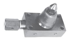
The Jergens Spring Loaded Work Jacks provide consistent support and rigidity to odd shaped workpieces. They are designed to prevent workpiece deflection under forces created during machining operations. Precision mated locking jaws grip the jackpost from both sides creating a vise-like action.
