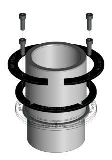
Square and triangle flanges designed for smaller diameter pins and bushings to conserve space
