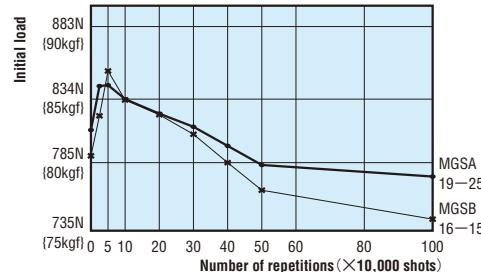
The load increases until approximately 300,000 shots due to friction between the rod and special urethane seal.
