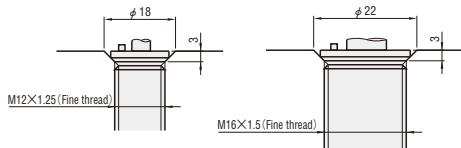
Prepare a tap hole for MGSA as shown above, so that the MGSA flange will be in close contact with the mounting surface.
