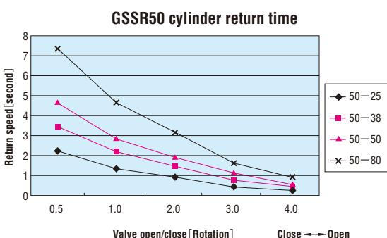
This graph shows the mean value from 10 piston rods. Use it only as a reference.
