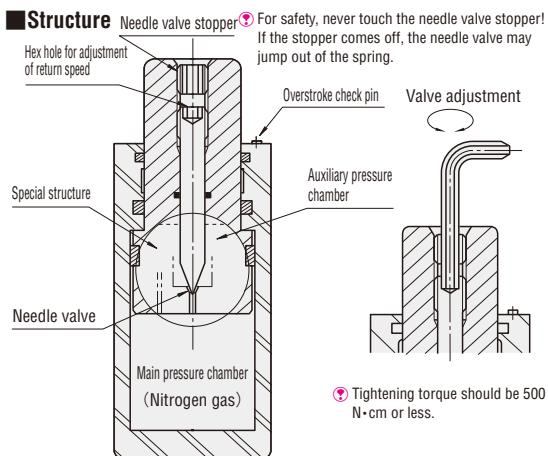
When the piston rod descends, nitrogen gas flows into the auxiliary pressure chamber.
