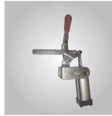
Pneumatic clamp with manual actuation handle
