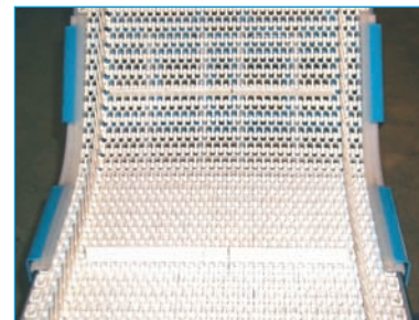
This is a photo of the hold down shoes at the lower curve.
