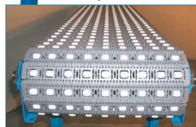
This is an end view photo of the 400 Roller Top Accumulation Belt.
