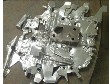
Ten hit pile-up destroyed the stripper window and caused major tooling repair.
