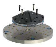
Mount to Fixture-Pro® base elements such as subplates via Jergens QLS Mounting System. A combination of (2) 12mm QLS shoulder screws and (2) M12 SHCS will accurately locate and securely clamp the pyramid to a base element.
