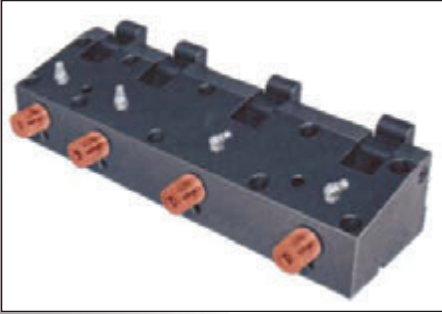
DESIGN A Four punches on a common horizontal centerline in an inboard cam unit.
