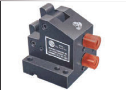
DESIGN D Two punches on a large, common vertical centerline. To assure smooth motion and prevent side loads, two triggers are used, one below and behind the other.
