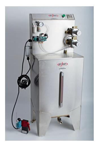
The MOD-1E-21 JET-SET® spray system comes standard with our 21 Gallon stainless steel tank with sight gauge, reusable filter, and air regulator. This system includes one JET-SET 9100 stainless steel piston pump (0-5cc per stroke) with 5 outlets for spray nozzles. The 9100 pumps are engaged using the electric solenoid to receive external signals for system activation. The MOD-1E-1 comes standard 110v unless specified.
