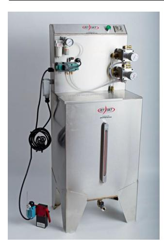
The MOD-1E-21 JET-SET® spray system comes standard with our 21 Gallon stainless steel tank with sight gauge, reusable filter, and air regulator. This system includes one JET-SET 9100 stainless steel piston pump (0-5cc per stroke) with 5 outlets for spray nozzles. The 9100 pumps are engaged using the electric solenoid to receive external signals for system activation. The MOD-2E-1 comes standard 110v unless specified.
