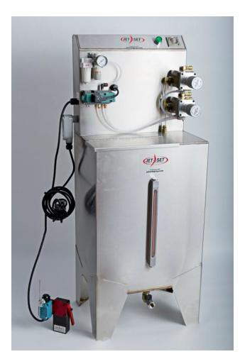
The MOD-2E-21 JET-SET® spray system comes standard with our 21 Gallon stainless steel tank with sight gauge, reusable filter, and air regulator. This system includes two JET-SET 9100 stainless steel piston pumps (0-5cc per stroke) with 10 outlets for spray nozzles. The 9100 pumps are engaged using the electric solenoid to receive external signals for system activation. The MOD-2E-1 comes standard 110v unless specified.
